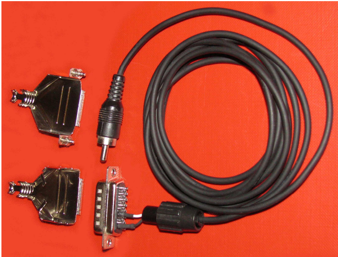
Photo 1. Original cable for VL-1000, DB15 connector disassembled. The two parts of the rear cover of the plug / socket. Band Data 2 connector (DB15) pins: connected only pin 9 and 11 (Original cable supplied with VL-1000). Photo by author.
